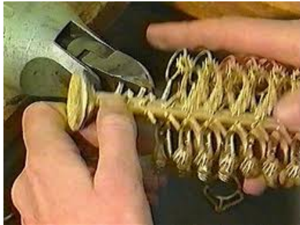
Modern lost wax casting method – screw tree
